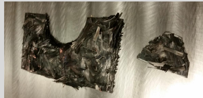
Flange Inserts “Tacked” for rapid molding
