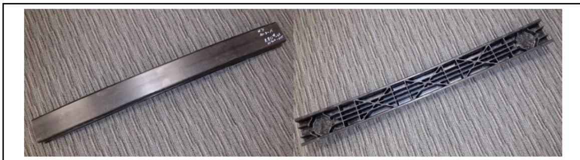
Figure 20. Left: Outside surface of the Front Bumper; Right: Inside structure of the Front Bumper
