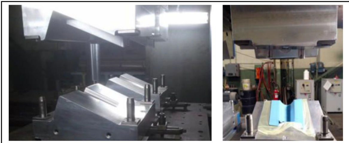
Figure 17. Left: Crush-can Preforming Dies. Right: Preformed crush-can in the dies
