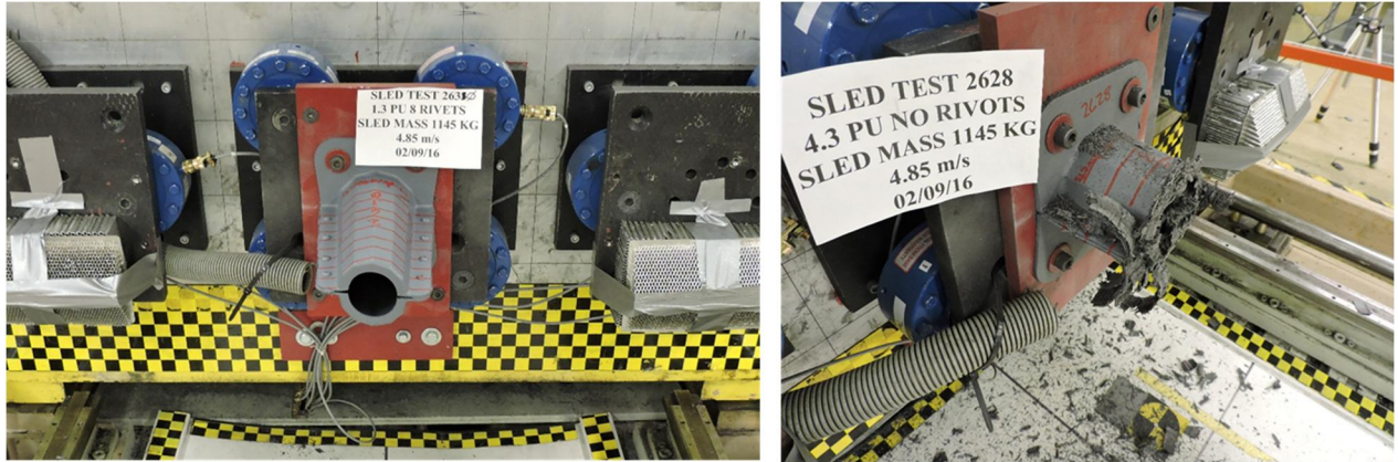
Figure 9: (Left) A crush can mounted on the wall prior to crash testing. (Right) The crush can after the test.
