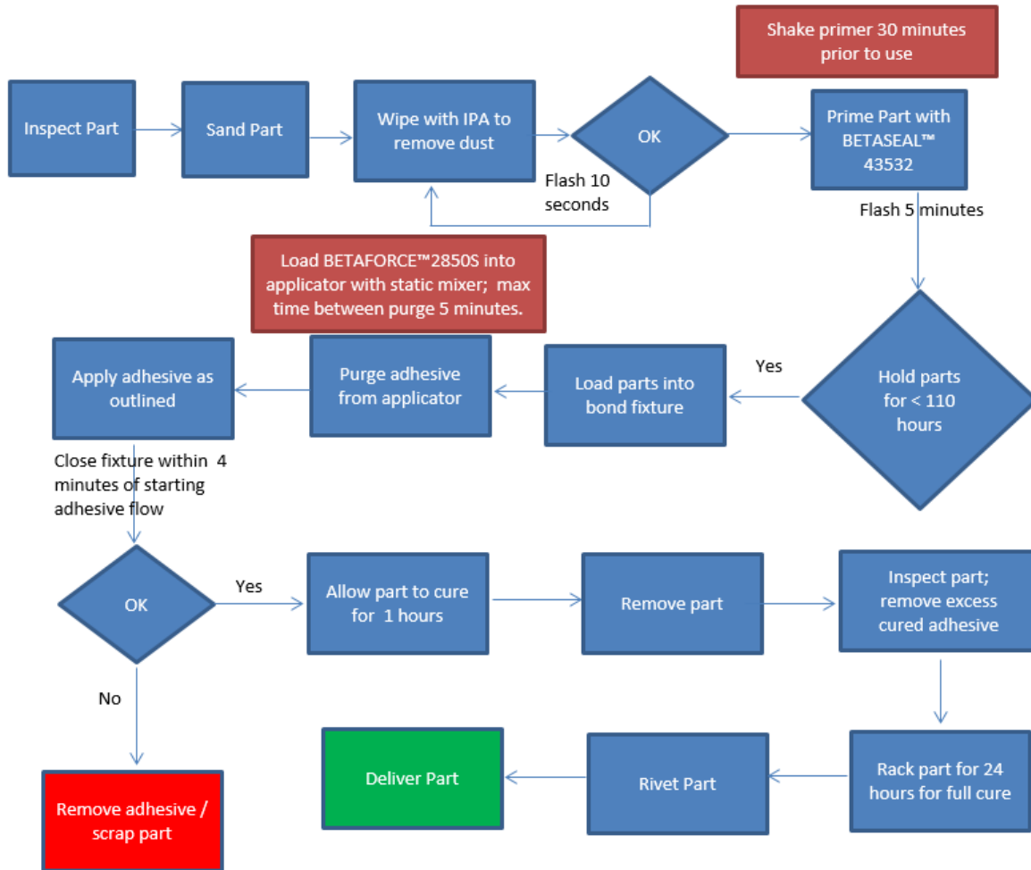
Figure 5: Flow chart of the bonding procedure for joining the crush can and bumper beam.
