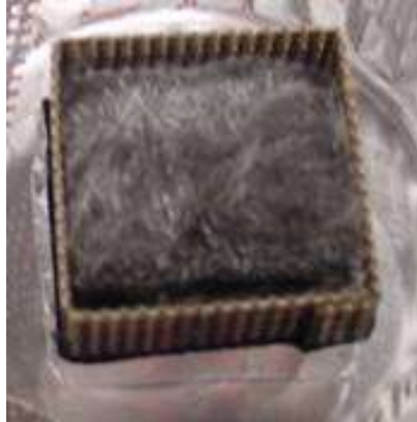
Figure 2. Aluminum form containing expanded mass of filaments after the first burn-off.
