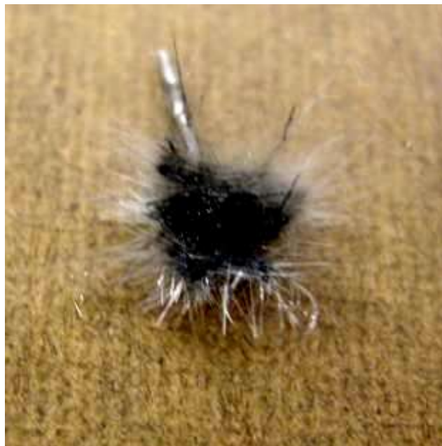
Figure 8. Extracted glass fiber-and-epoxy specimen
