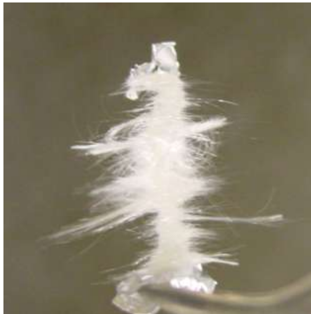
Figure 6. Extracted glass fiber-and-epoxy “plug” specimen
