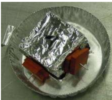
Figure 7. Hypodermic needles inserted in the fiber mass at pre-determined locations.
