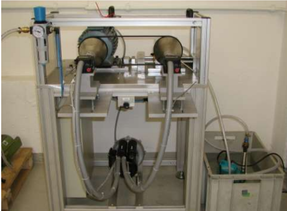
Fig. 10: Test bench for a belt pulley [20]
