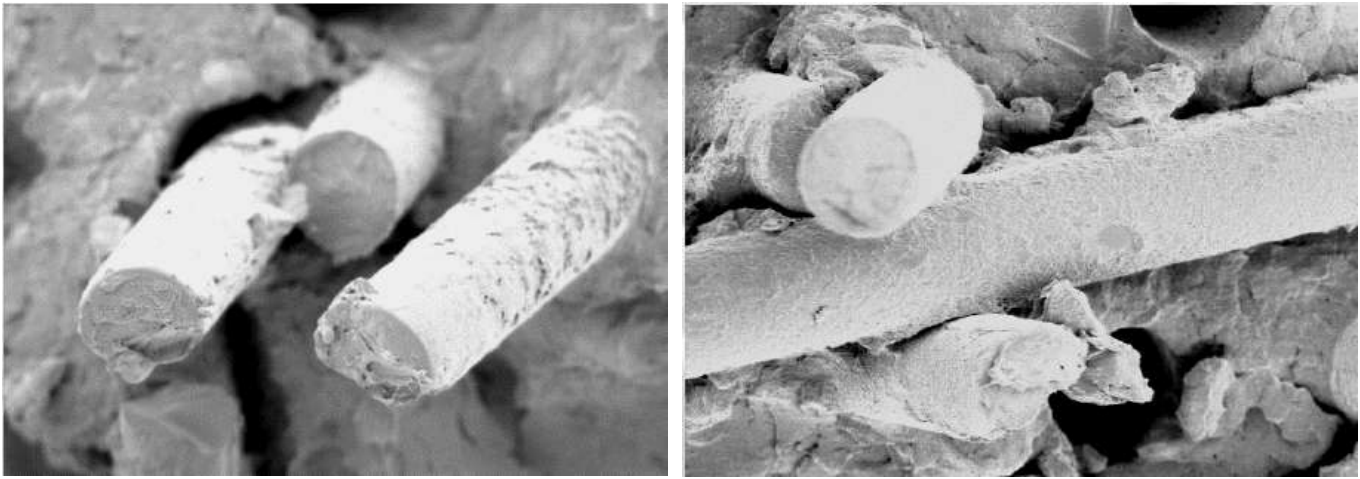
Fig. 1: SEM micrograph of the fracture surface of a short specimen of PA 6T/6I-GF40MX2
