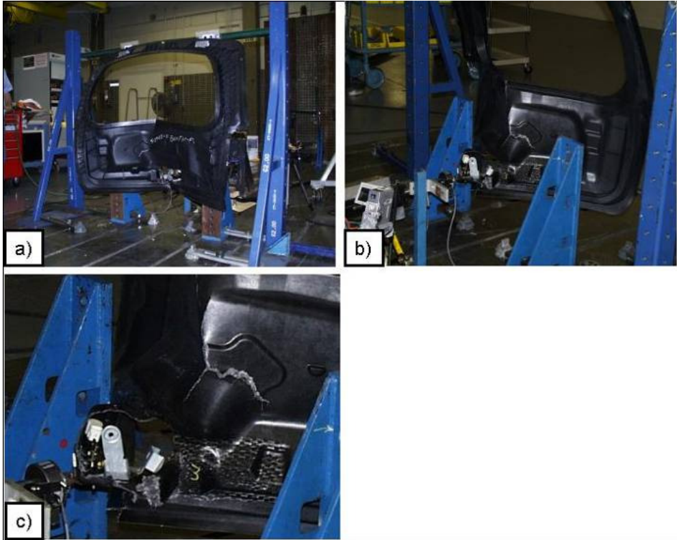
Figure 15. Various views of the GMTEX reinforced GMT inner panel while still under load at maximum displacement of 264 mm.
