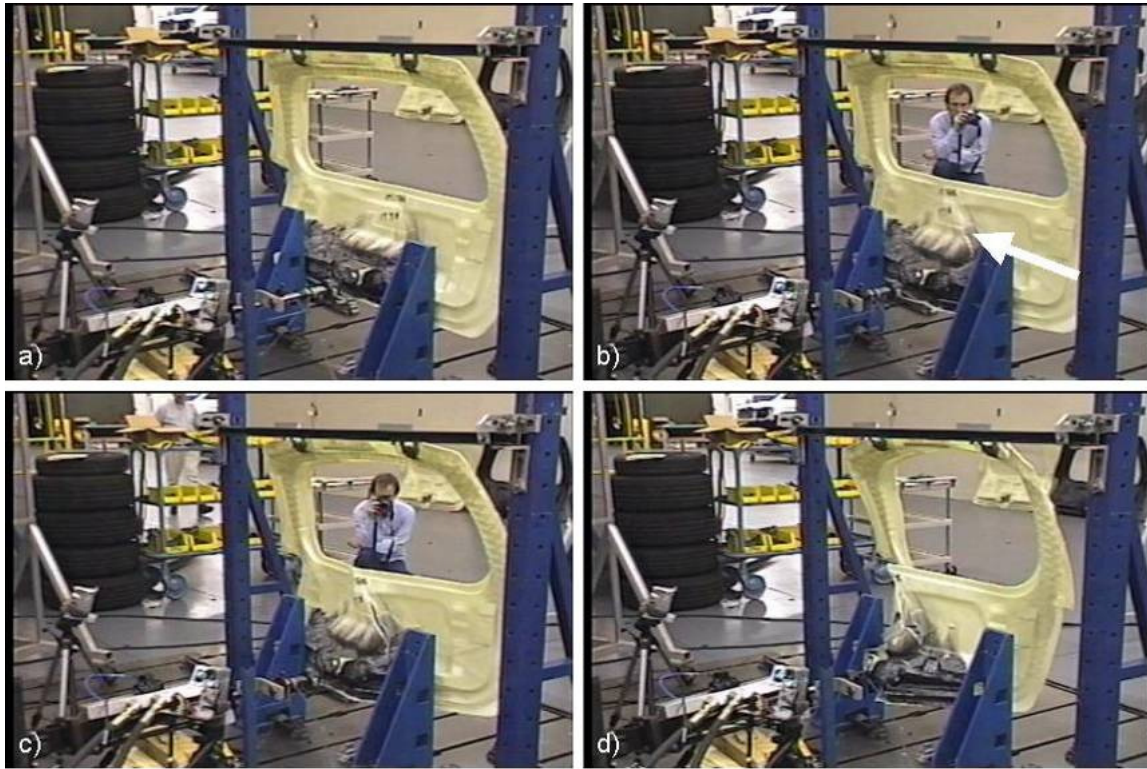
Figure 14. Twintex reinforced DLFT inner panel load displacement test showing a) initial state, b) first crack appearance, c) complete cracking of the unreinforced portion and d) maximum displacement of 270 mm.
