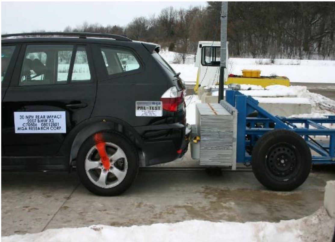
Figure 2. FMVSS 301 offset deformable barrier test configuration[2].
