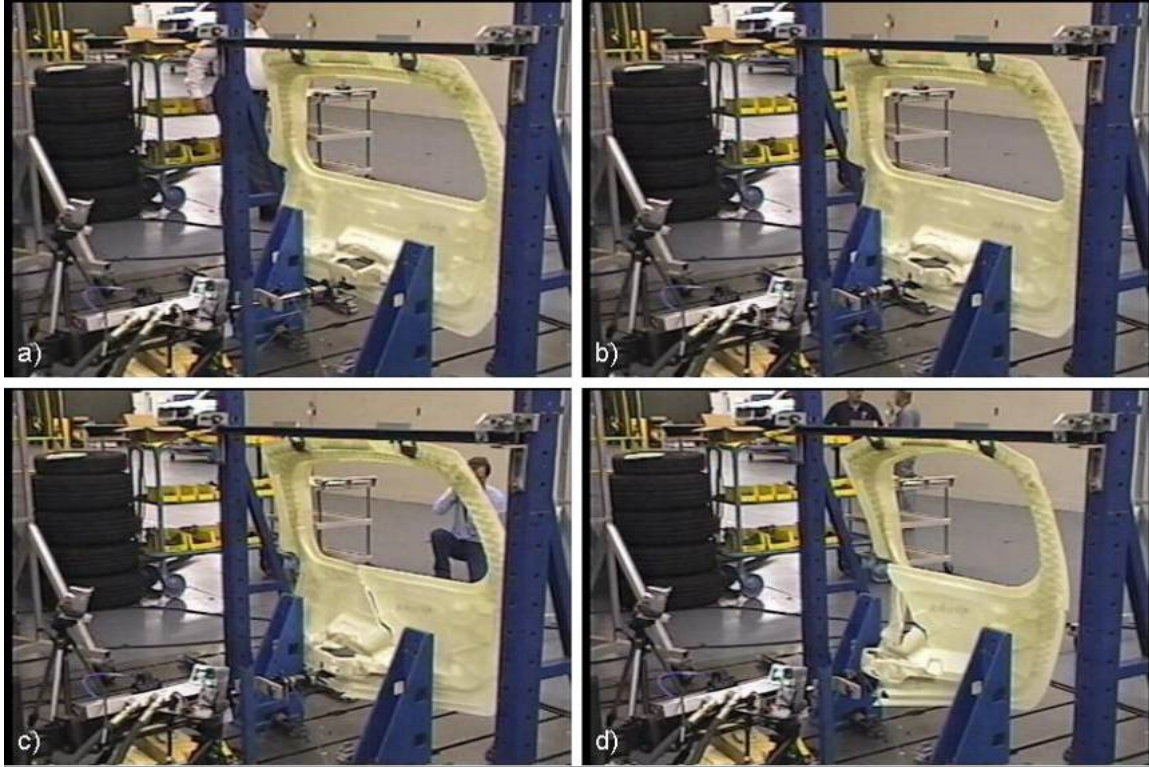
Figure 17. Hardwire reinforced DLFT inner panel load displacement test showing a) initial state, b) first crack appearance, c) complete cracking of the unreinforced portion and d) maximum displacement of 266 mm.
