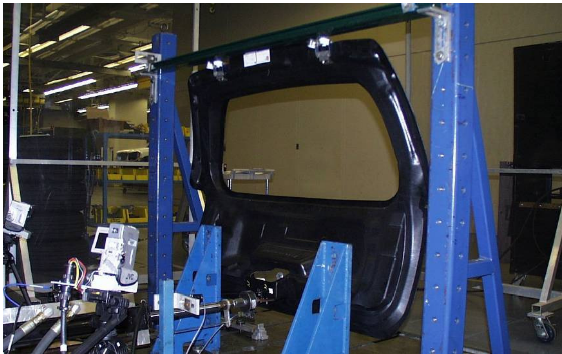
Figure 10. Experimental setup at the GM Body Test Lab for measuring the load-displacement response of a liftgate when the striker is pulled forward (in-car direction).
