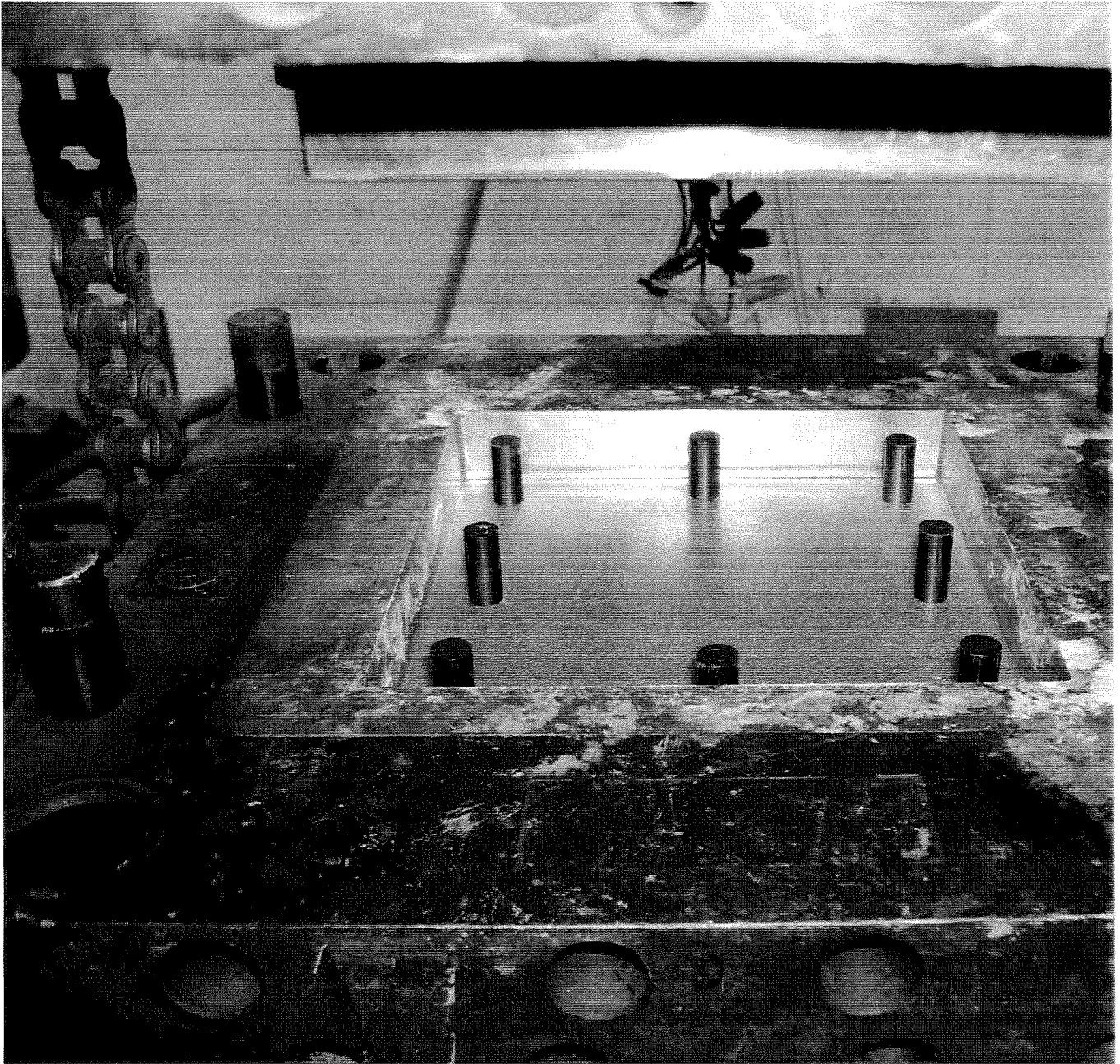
Figure 1: Compression mold for a plaque. Tool temperature at 300 deg F
