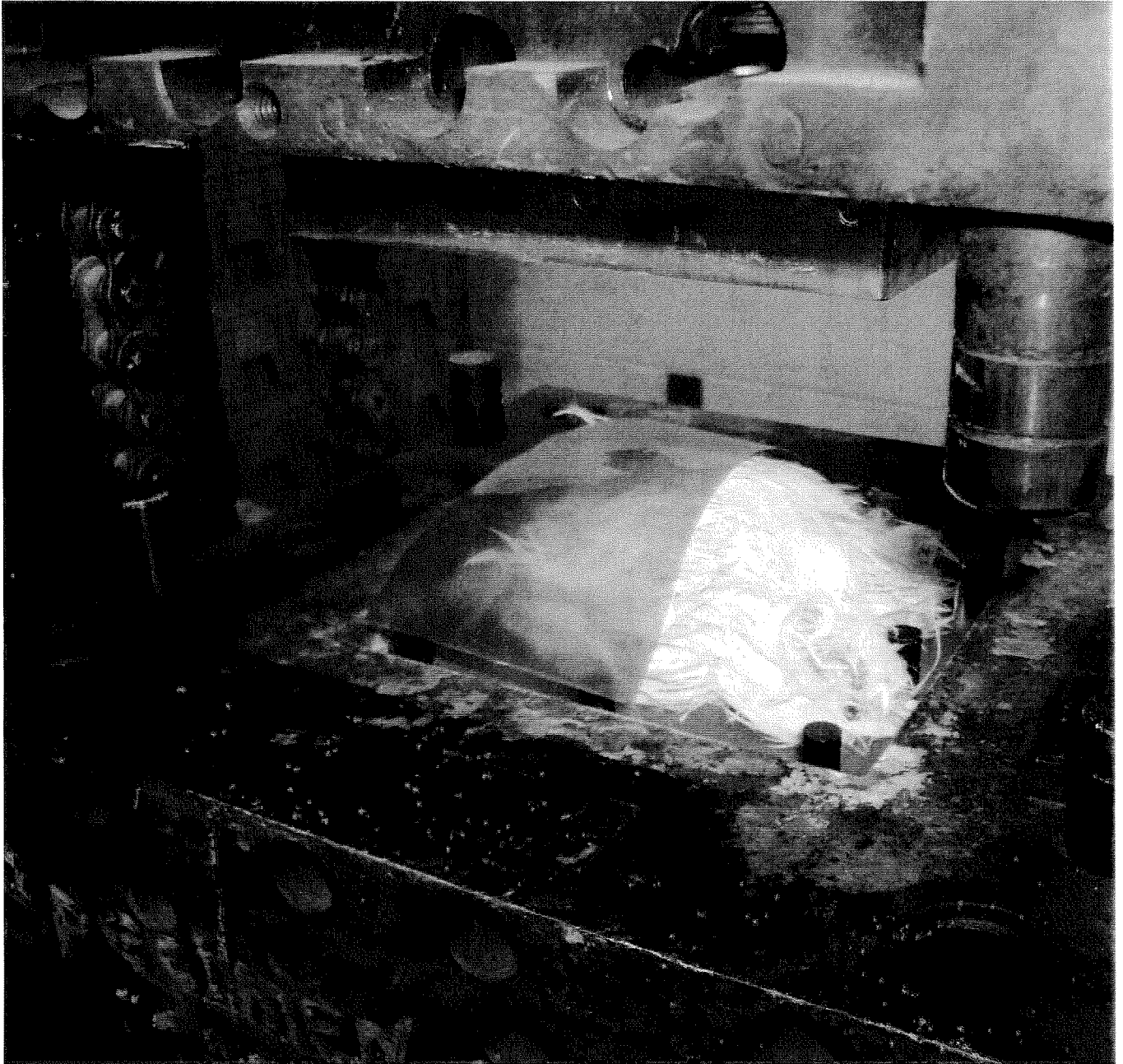
Figure 3: Compression mold with BMC compound and the FTHC with a wood grain image. The Film is oriented in a manner in which the coated/printed side of the film is in contact with the BMC compound.
