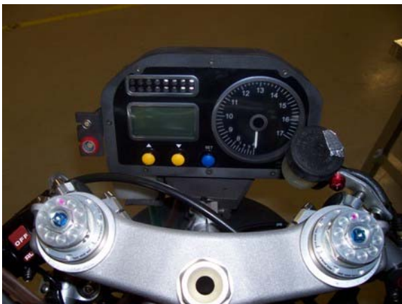
Figure 4 – The new Windform XT dashboard made by SLS on the bike: it is an all-in-one ECU, DATALOGGER and CONTROLLER box
