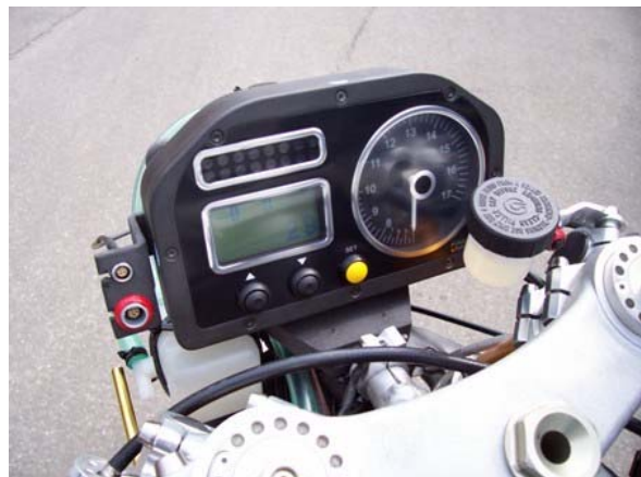
Figure 4 – The new Windform XT dashboard made by SLS on the bike: it is an all-in-one ECU, DATALOGGER and CONTROLLER box
