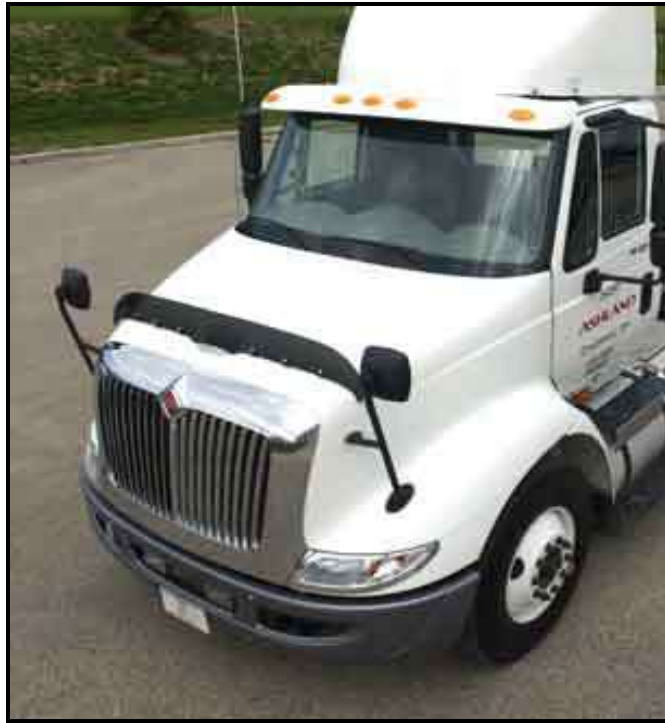
Figure 3. Completed low mass SMC hood assembly on fleet vehicle.
