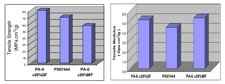
Figure 6: Comparison of the specific tensile strength and modulus (relative to density) of 20% curauá fiber filled PX07444 with 20% of glass fiber (GF) or talc (MF) reinforced PA-6.
