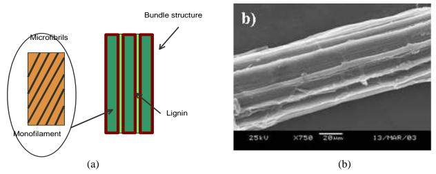
Figure 2: a) Structural model of the natural fiber and b) Micrograph obtained by SEM of the curauá fiber surface
