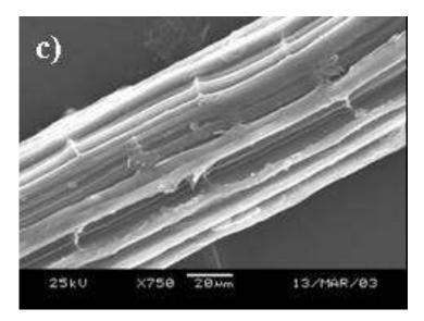
Figure 5: SEM micrograph of curauá fibers surface after alkaline treatment.
