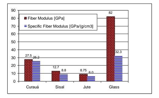
Figure 4: Comparison of the tensile modulus (nominal and specific) of natural fibers with glass fiber
