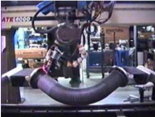
Automated Dynamics – Fiber Placement
