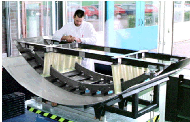
Figure 1. Composite-intensive energy-absorbing subfloor of commuter aircraft [7]
