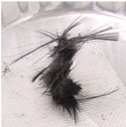
Figure 5. Carbon fiber and epoxy plug.
