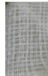
GMTex grades with 1/1 reinforcement weave
