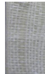
GMTex grades with 1/1 reinforcement weave
