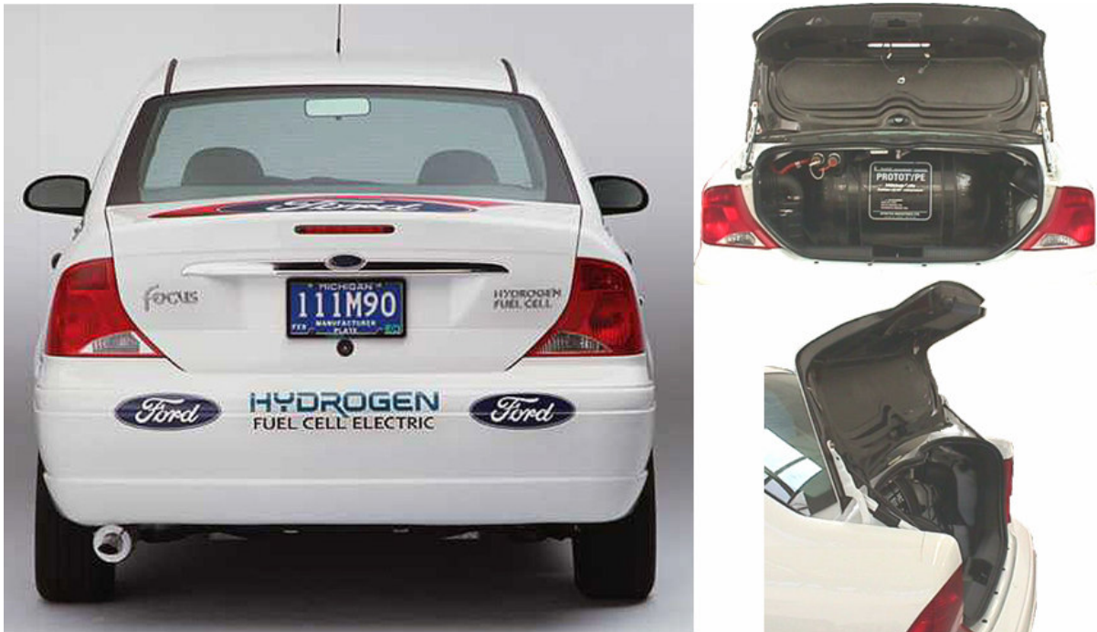
Figure 19: Installed Decklid Assembly (Ford Motor Company)
