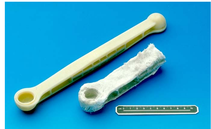
Enhanced picture of an injection molded part before and after being burned off (the white part represents the glass fiber matrix)
