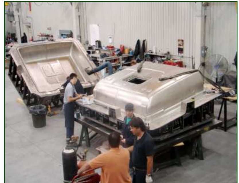
Assembly of Nickel Shell to Mold Base
