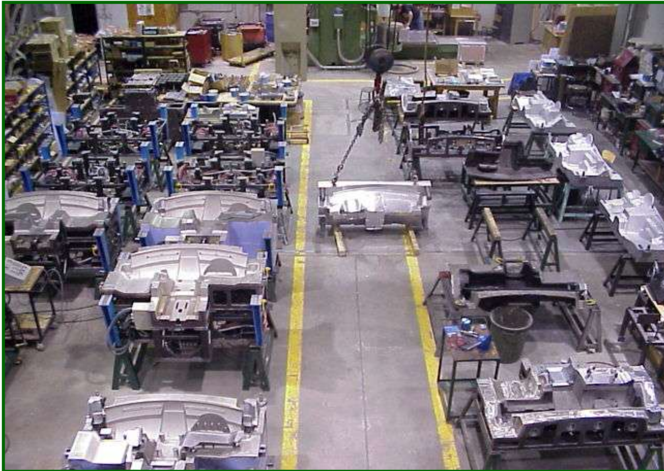
DIRECT BACKFOAM IP MOLD BUILD
