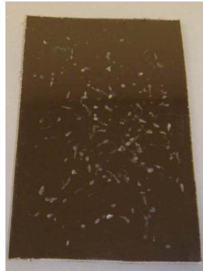
Figure 6: Heavy Marring on Test Specimens
