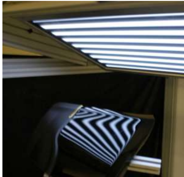
Figure 6. Distortion of a Reflected Grid as Seen on a Bumper.
