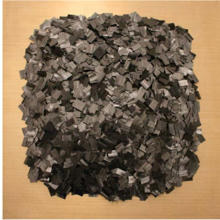
Figure 2. Random distribution of prepreg chips before curing.
