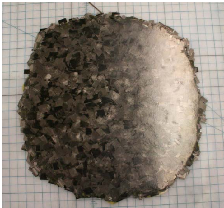
Figure 3. Random distribution of prepreg chips after curing, forming a raw laminate.
