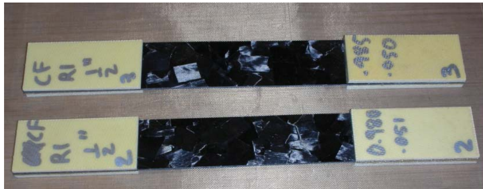
Figure 7. Typical tensile test specimens with glass fiber/ epoxy tabs.
