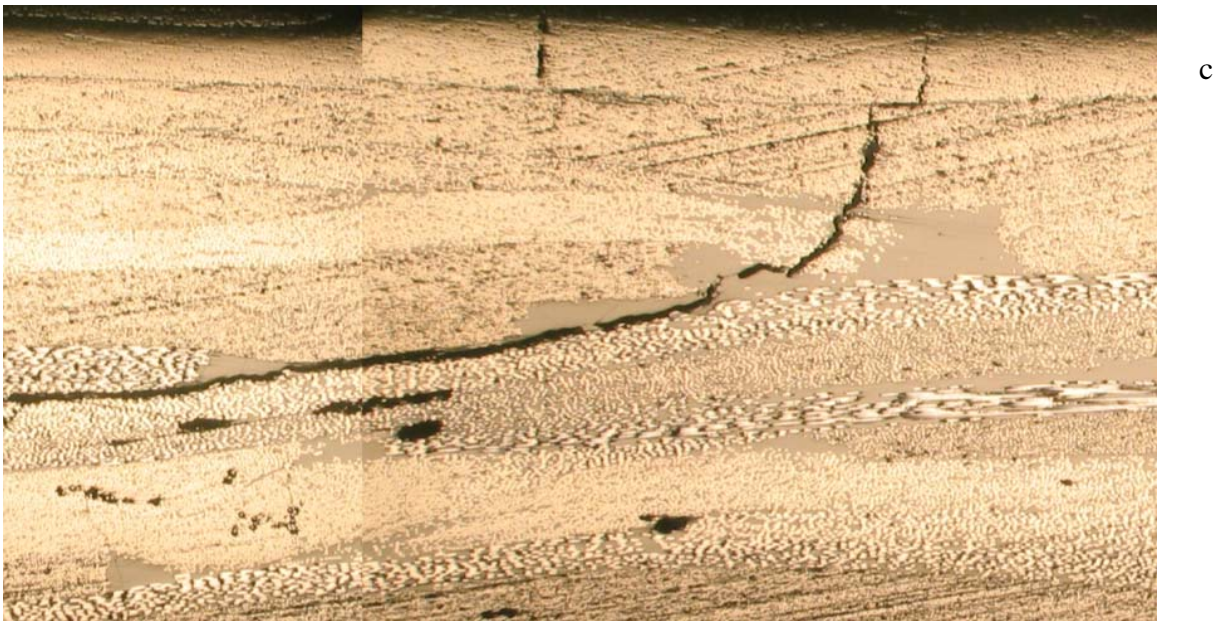
Figure 11 a-c. Sequence of micrographic pictures at increasing magnification of typical tension failed specimen, secondary failure.
