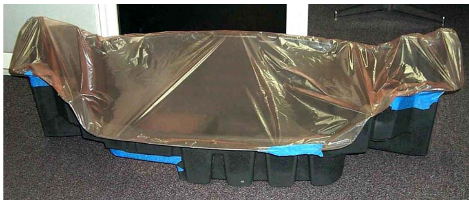
Figure 2. A trunk pan sealed with SMC carrier film to monitor styrene concentration over time using an IR detector.
