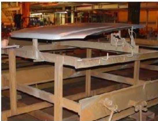
Figure 4. Mule used to carry SMC hoods through E-coat process at Shreveport paint shop.
