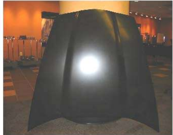
Figure 1. A molded Corvette C6 hood made with experimental SMC.
