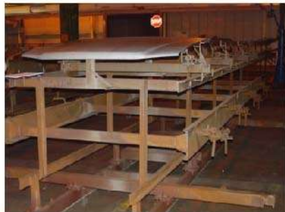
Figure 4. Mule used to carry SMC hoods through E-coat process at Shreveport paint shop.
