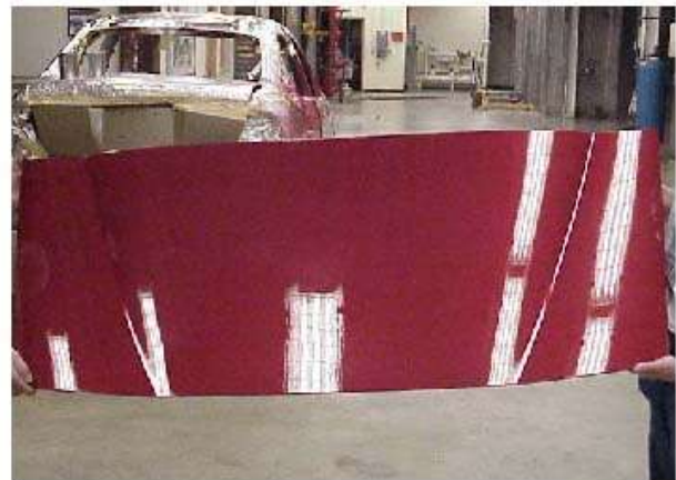
Figure 2. A molded Corvette C6 quarter panel and a decklid made with experimental SMC
