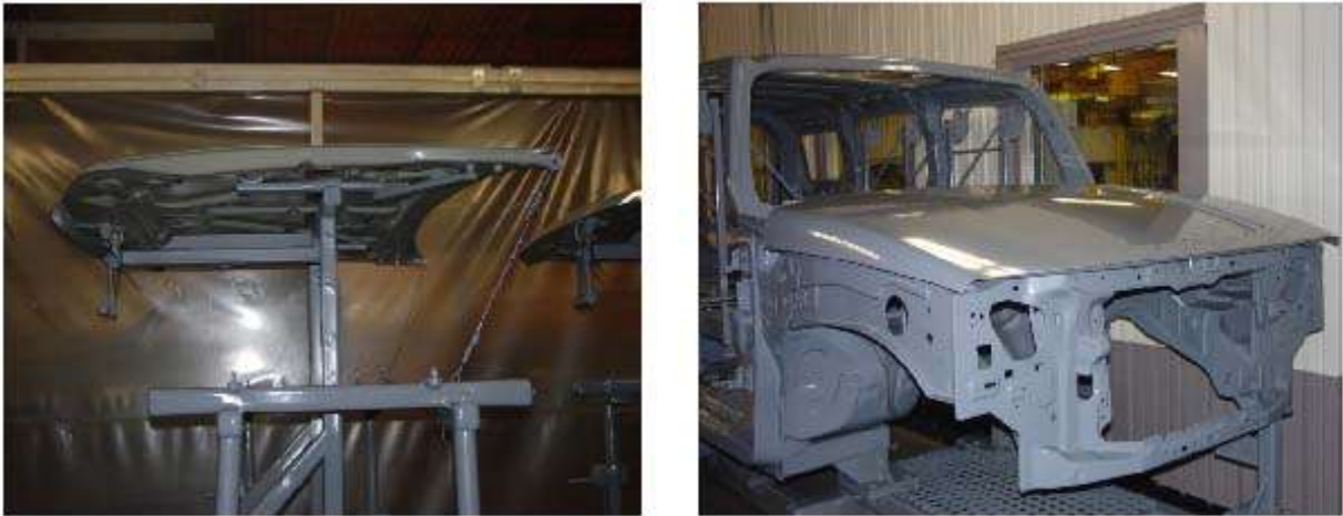
Figure 5. Mules used to carry SMC hoods through powder and top-coat application process at Shreveport paint shop.
