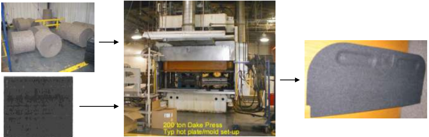
Figure 6: Raw flax/PP and carpet, through hot plate / cool form tool, to final carpeted panel.
