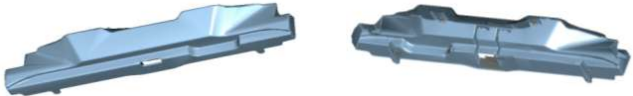
Figure 9: Front and rear views of the upper reinforcement.
