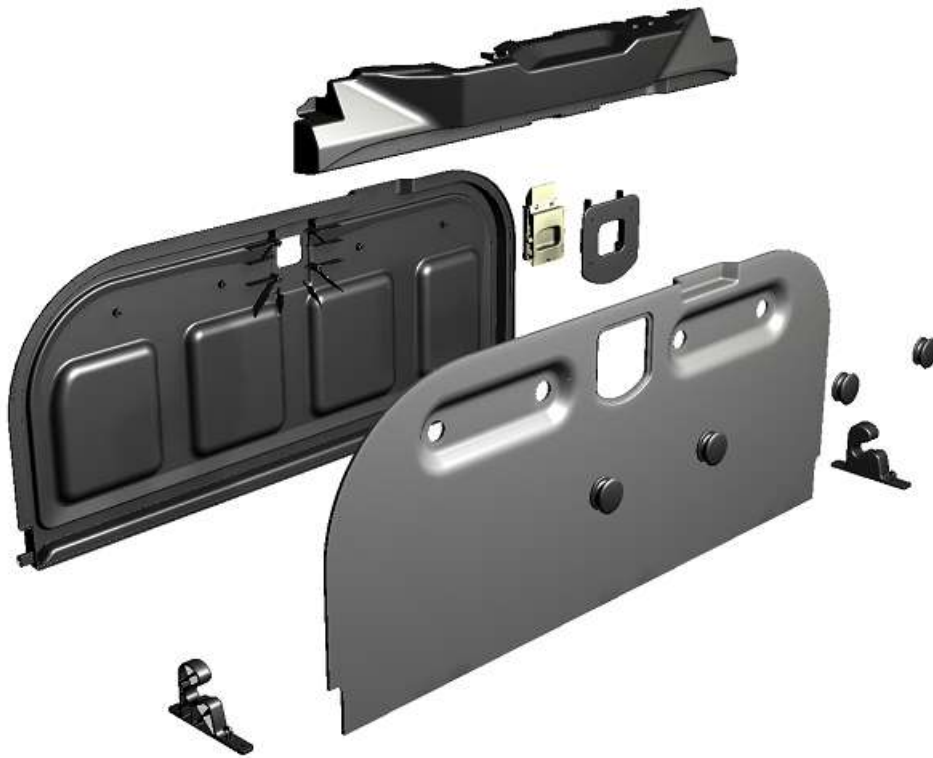
Figure 3: Exploded view of divider assembly (including upper reinforcement and hinges).
