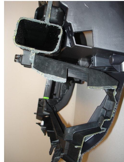
Side View of I/P Structural Duct
