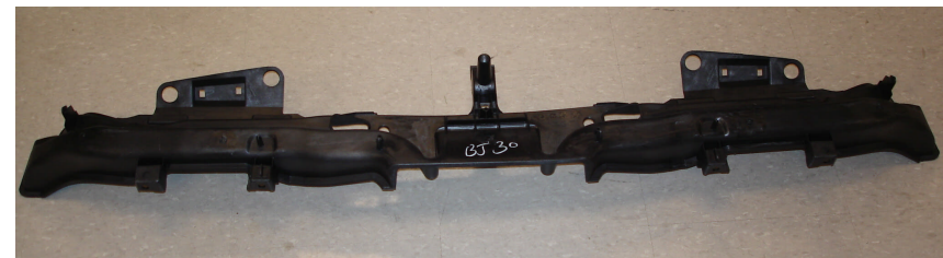
Front View of I/P Structural Duct
