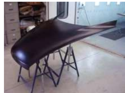
Figure 16c. Completed hood assembly with matt black topcoat.
