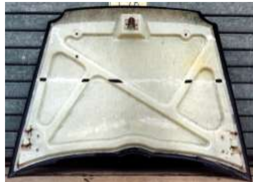
Figure 2b. The compression-molded chopped-fibre reinforced thermoplastic frame of the hood for the Vector II concept car (shown following a front barrier collision test)
