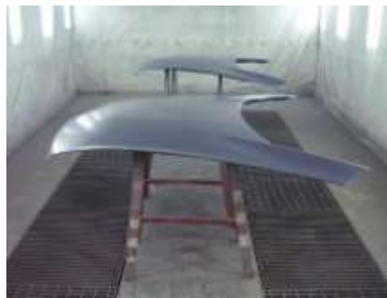
Figure 16b. Hood assemblies with primer coat applied.
