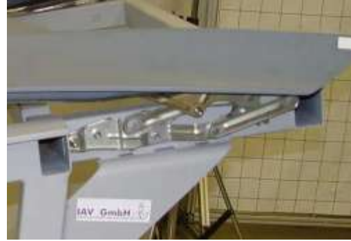
Figure 17b. Close-up detail of hinge attachment to support frame.
