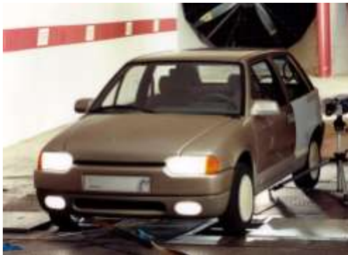
Figure 2a. The Vector II concept vehicle developed by GE Plastics in Europe during the late 1980's featured an all-thermoplastic hood.
