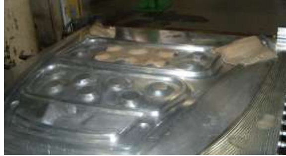
Figure 11b. Aluminum tool core for hood inner frame.
