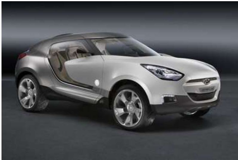
Figure 3: The Hyundai HED-4 QarmaQ advanced technology demonstration vehicle features a prototype hood made using HPPC technology.
