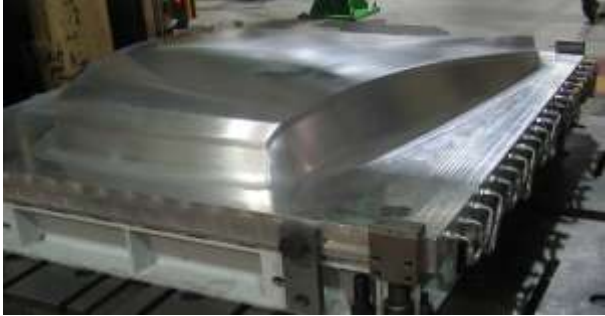
Figure 11a. Aluminum tool core for hood outer skin.
