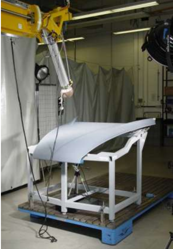
Figure 17a. Overall view of the impact testing set-up showing the hood assembly mounted on the support frame, impactor launcher and laser measurement device.
