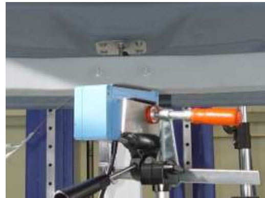
Figure 17c. Close-up detail showing the laser distance-measurement apparatus positioned under the hood to measure intrusion into the engine bay.
