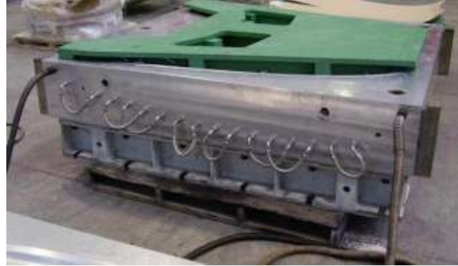
Figure 15b. A hood assembly curing with the pressing frame holding the parts in place in the cavity half of the outer skin tool.
