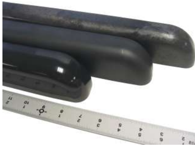
Figure 12: Molded part shown top to bottom: 20% ASA LFRT molded at conventional temperatures; 20% ASA LFRT molded with Heat and Cool in unpolished tool; 20% ASA LFRT molded with Heat and Cool in polished tool
