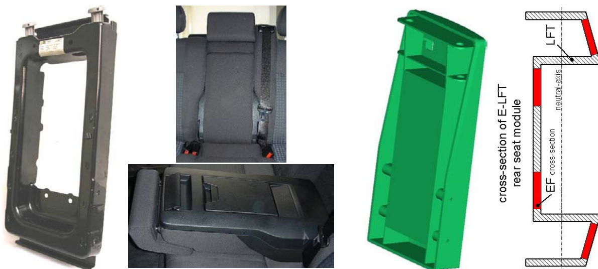
Figure 13: Rear seatback module : (left) steel version and complete module, (right) E-LFT part with cross section
