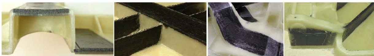
Figure 4: Possibilities of EF tape design freedom, EF is colored black, LFT natural
