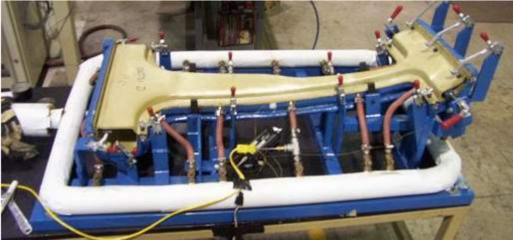
Figure 15. Part with inner placed on top of outer in bonding position; clamps in closed position
