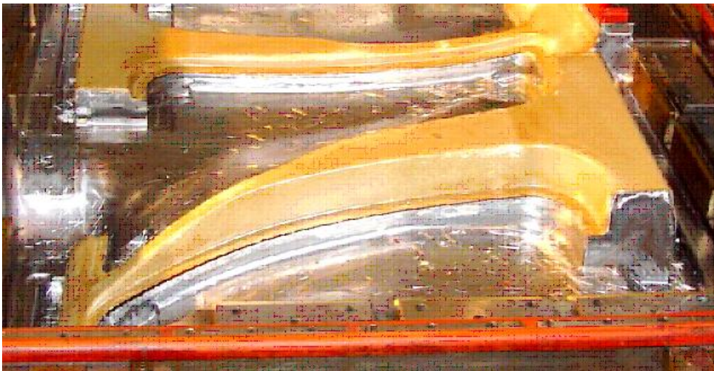
Figure 10. Molded B-pillars in the lower mold half.
