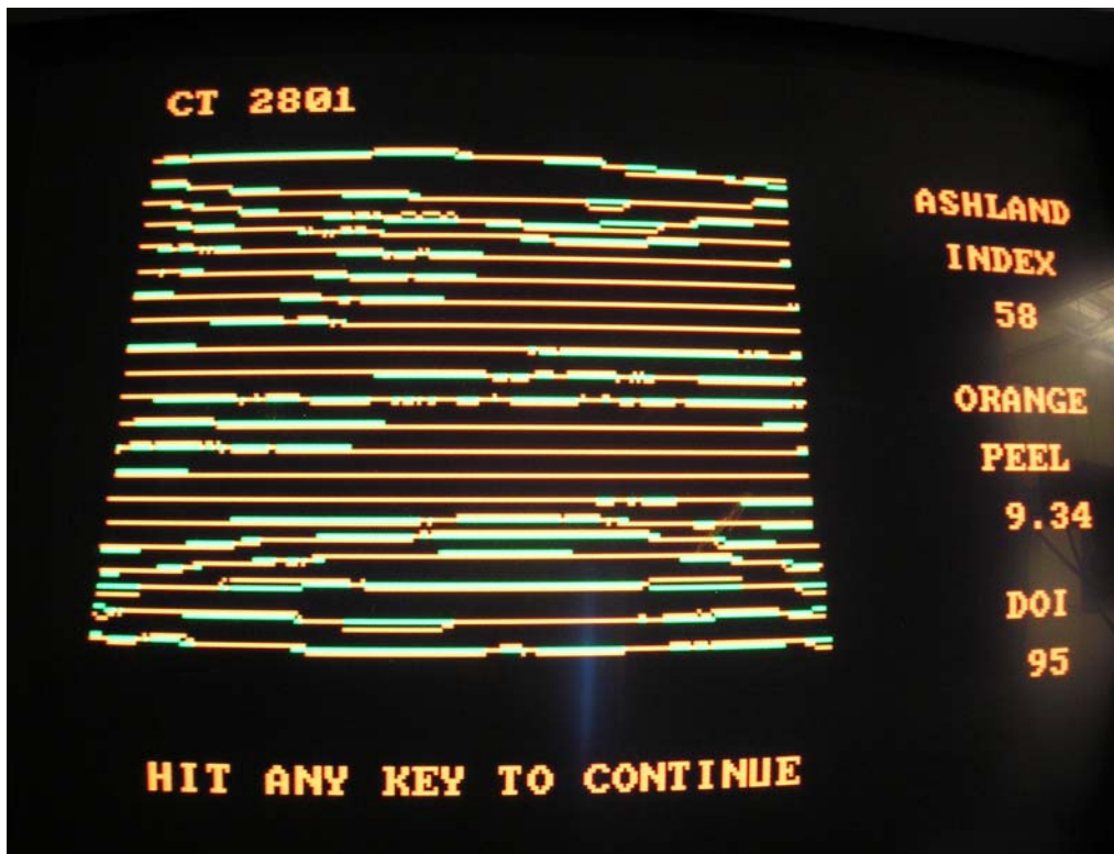
Figure 4: Loria® class-A SMC surface waviness test results
