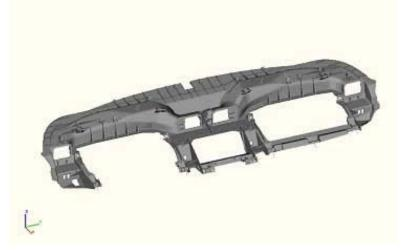
Figure 4: The upper IP frame is injection molded from LFT polypropylene with 40% long-glass fiber reinforcement. The lower IP carrier is subsequently vibration welded to the upper IP frame.
