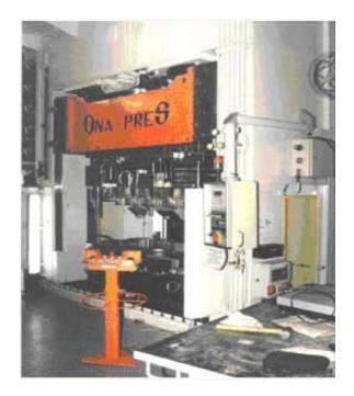
Figure 9: Vertical compression molding press for production of the IP carrier ...
