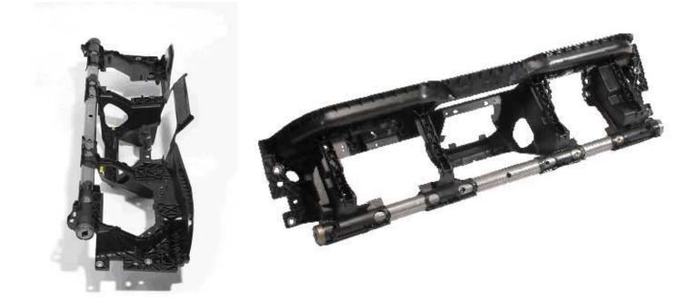
Figures 14 & 15: It was very important to maintain strong knitlines at junction points between the CCB and the GMT carrier. This was accomplished by careful control of process parameters, particularly pressure.
