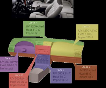
Weathering SAE J 1885 Impact Scratch Heat Chemical
