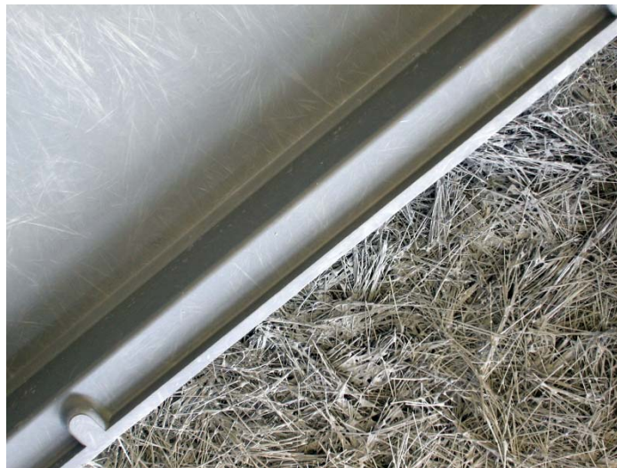
Figure 2. Finished Part on Upper Half and Interwet Laydown on Lower Half
