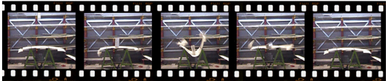
Figure 7. Impact trials sequence 5 . (36 kg falling from a height of 3.25 m). On the surface, some signs and abrasions remain present but easily recoverable).
