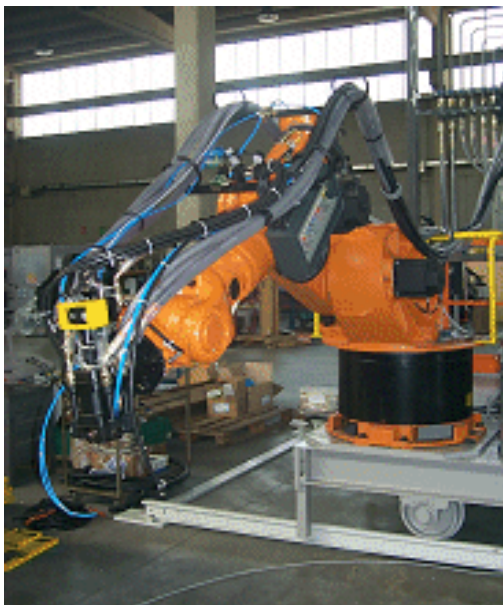
Figure 3. Interwet Mixhead and Chopper Mounted on 6-Axis Robot
