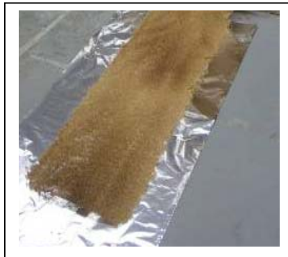
Figure 2. Semi-consolidated biocomposite sheet produced from SMC processing
