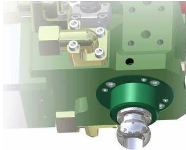
Figure 3: The front end of the discharge tube and the spherical end of the cleaning piston are washed after every shot to remove material residues.
