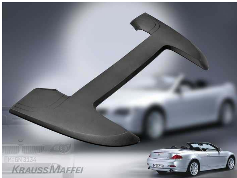
Figure 7: To produce automotive components with a grained surface, the substrate is molded in a LFI-PUR® process then flooded with a PU skin.
