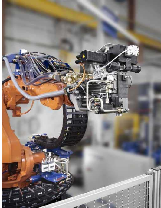
Figure 1: At the heart of the process – the LFI process mixing head.
