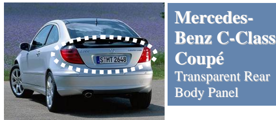
Figure 14: Mercedes-Benz C-Class Coupé PC transparent rear body panel
