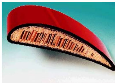
Figure 8: Paint film over composite polyurethane for class-A surface
