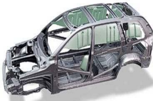
Figure 6: PMH side airbag system with TPU sleeves in the energy management tubes packaged in the roof framework
