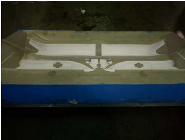
Figure 7: 6-cavity mold for Ford GT – Photo courtesy of WK, Industries, Warren, MI
