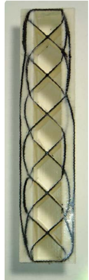
Demonstrator: LFT-PP/GF combined with continuous fiber structure
