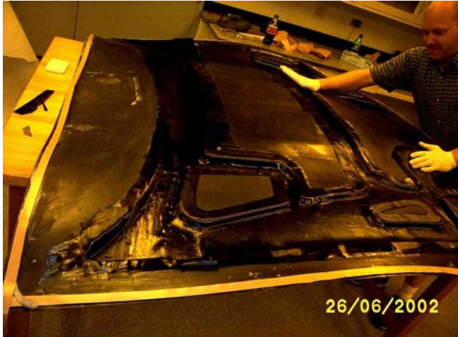
Figure 1. Hood inner fabrication
