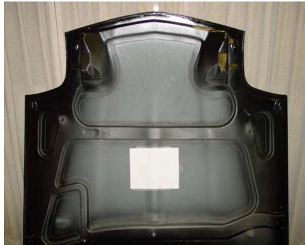
Figure 4. Finished hood inner
