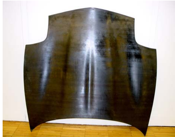
Figure 6. Electron beam cured corvette hood outer
