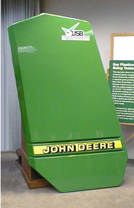
Figure 10: The first John Deere Round Hay Baler panel made with triglyceride-based resins.
