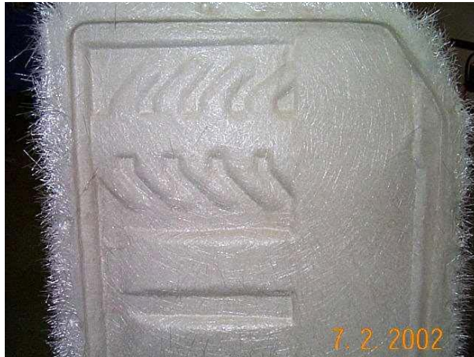
Figure 12. Photo showing a high-solids prepreg based on the oligomers following thermal-spray processing but before compression molding.
