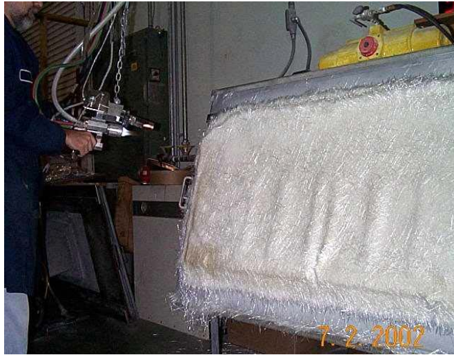
Figure 11. Photo showing the final stages of the thermal spray process for manufacture of a large prepreg component.
