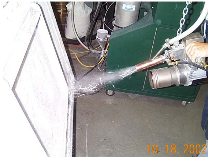
Figure 10. Photo showing the co-mingling of oligomers and glass fiber during the thermal spray process for prepreg manufacture.
