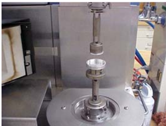
Figure 5. Photo of the cup-and-plate fixtures in the rheometer sample chamber.
