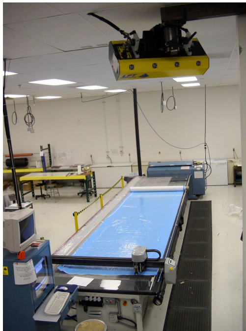
Figure 7: Autometrix CNC cutting table with LPT Inc. laser projection head above
