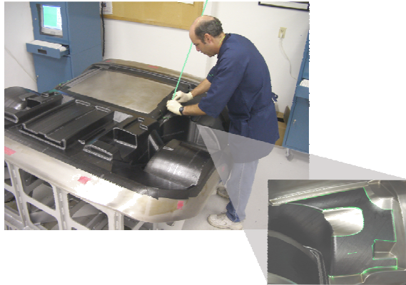
Figure 8: Lamination with laser projection
