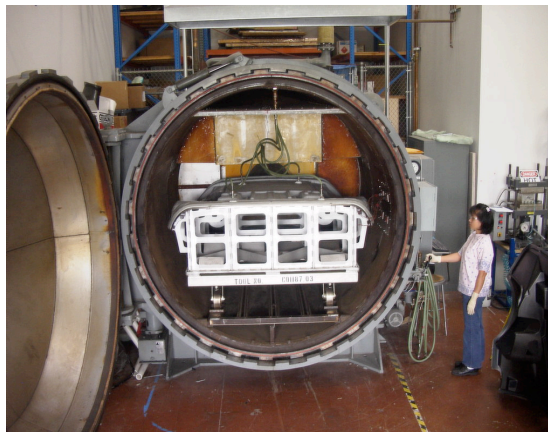
Figure 9: Mold in autoclave with vacuum connected
