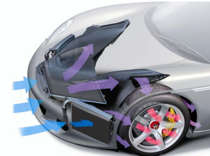
Figure 5 Cooling air routing
