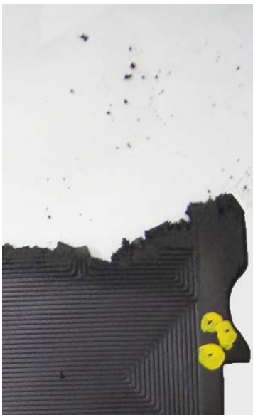
Figure 8: Mold filling during short shot and simulation.
