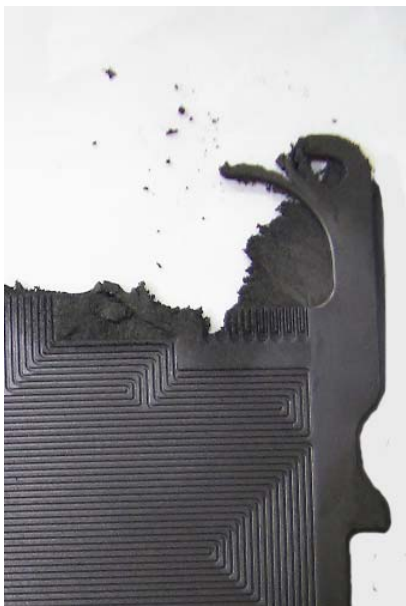
Figure 10: Mold filling during short shot and simulation.
