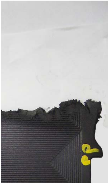
Figure 7: Mold filling during short shot and simulation.
