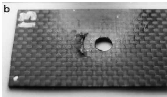
Figure 1. Re-plot from Figure 6(b) of Ref. 11: damage at washer edge for bolted joint
