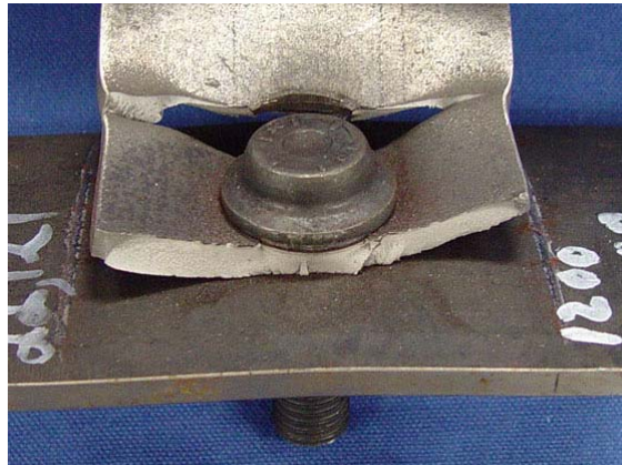
Figure 6. Fatigue failure modes for steel/steel joints
