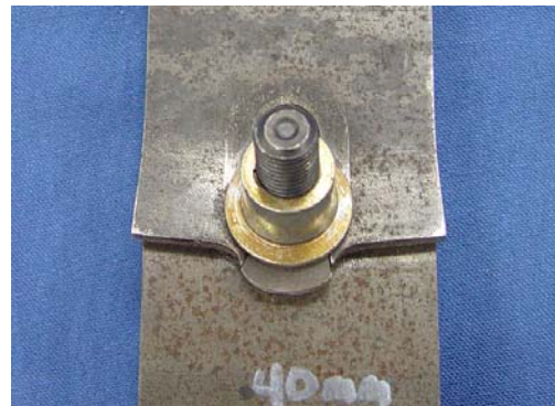
Shear out of sheet through edge margin
