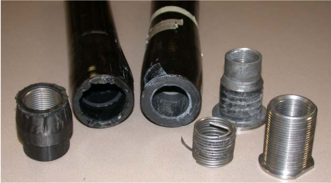
Figure 7. Various end inserts and tube ends tested during development. Note the step in the tubes indicating the presence of an inner tube used instead of tooling / mandrel during roll wrap and consolidation.
