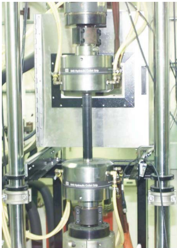
Figure 3. Durability testing of end inserts – ORNL MTS machine. This MTS machine also used for ultimate buckling load test. (Courtesy of ORNL)
