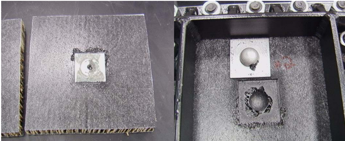
Figure 3: Embedded inserts geometry and placing.
