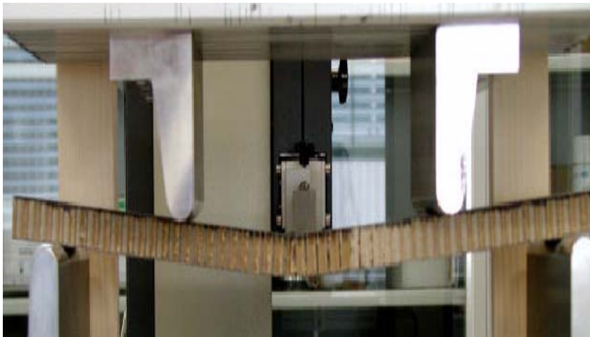
Figure 8: 4-Point Bending Test
