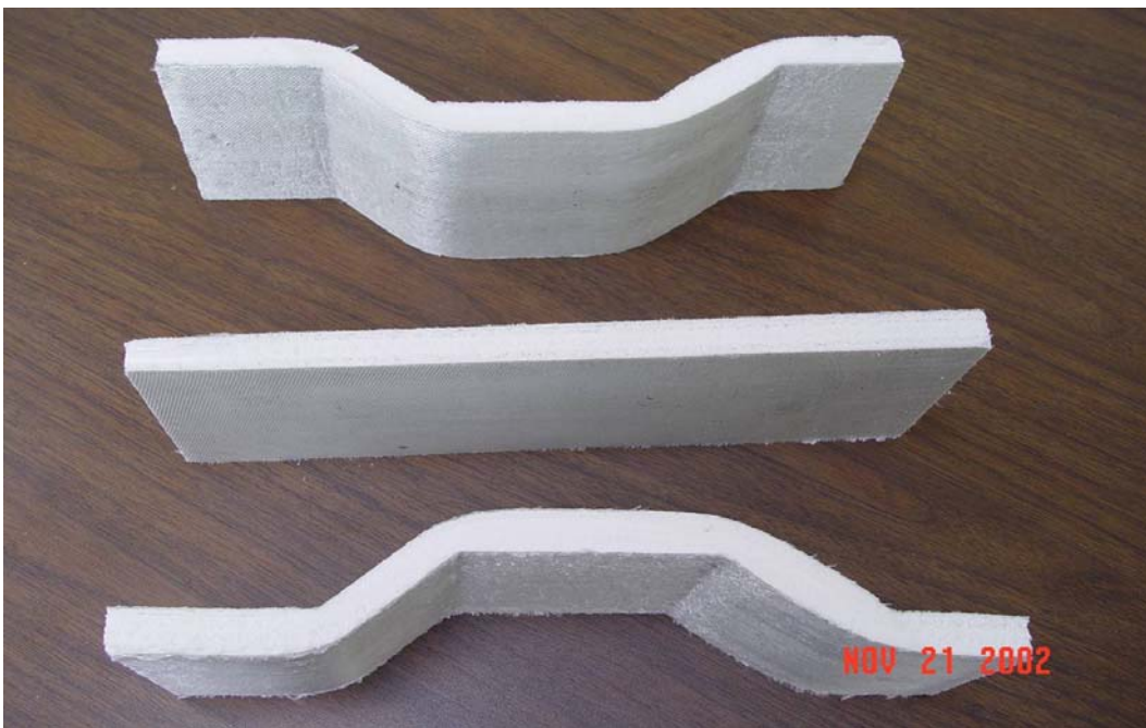
Figure 31. Thermoplastic Composite Sandwich of E-Glass/ PET Facings & CS-PET Foam Core, Before and After Thermoforming
