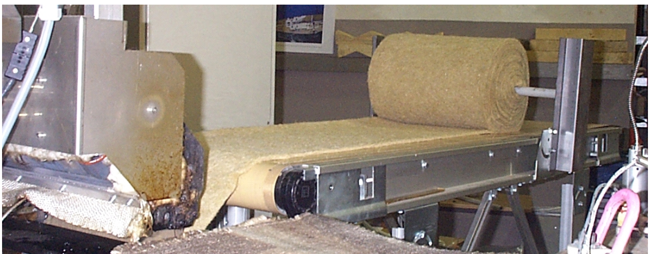
Figure 4a: Dosing of natural fiber mat – conveyer-belt
