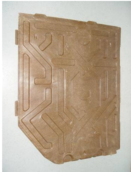
Figure 6: Underbody cover of Mercedes A-class
