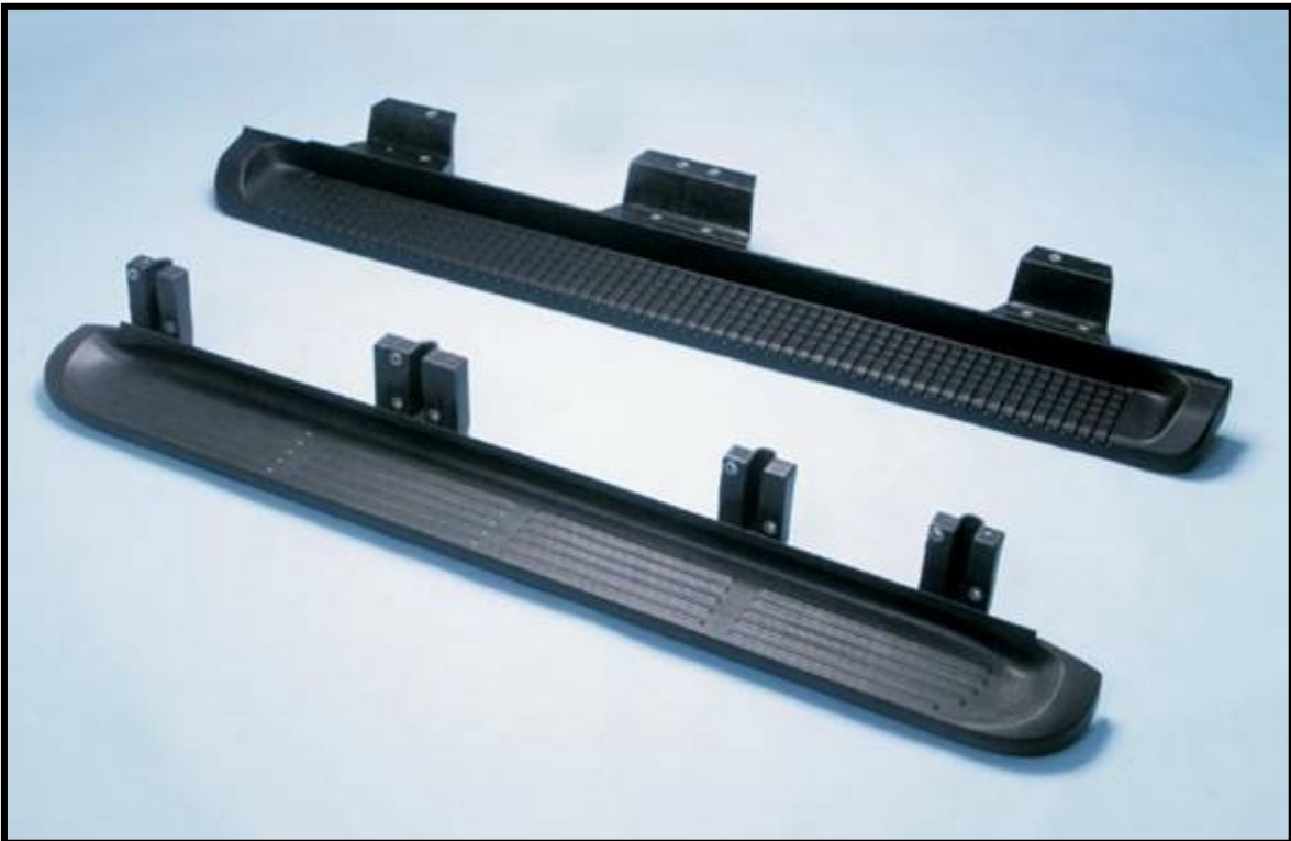
Figure 4: Ford F-150 and Ford Explorer production one piece composite running boards
